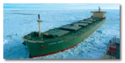
For the first time ever, an ice class 1A bulk carrier "Nordic Orion" 225 m long from the Nordic Bulk Carriers A/S Danish company, is using the North West Passage in September 2013 as a transit trade lane when transporting 75000 tons of coal from Vancouver, Canada to the port of Pori in Finland
